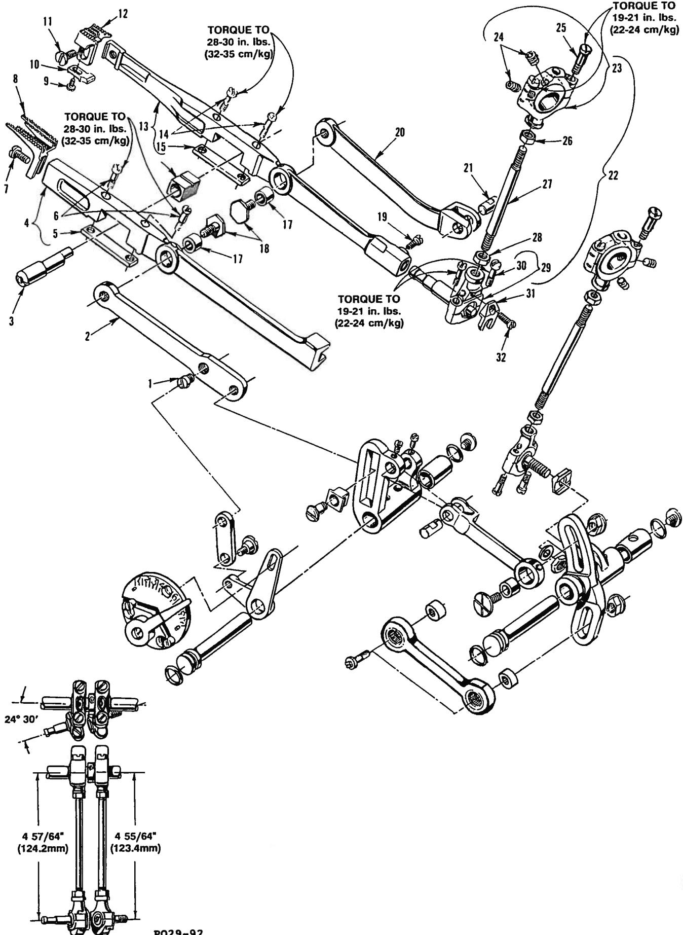
**DIFFERENTIAL & MAIN FEED BARS, FEED DOGS & FEED LIFT ECCENTRIC ASSEMBLY**
