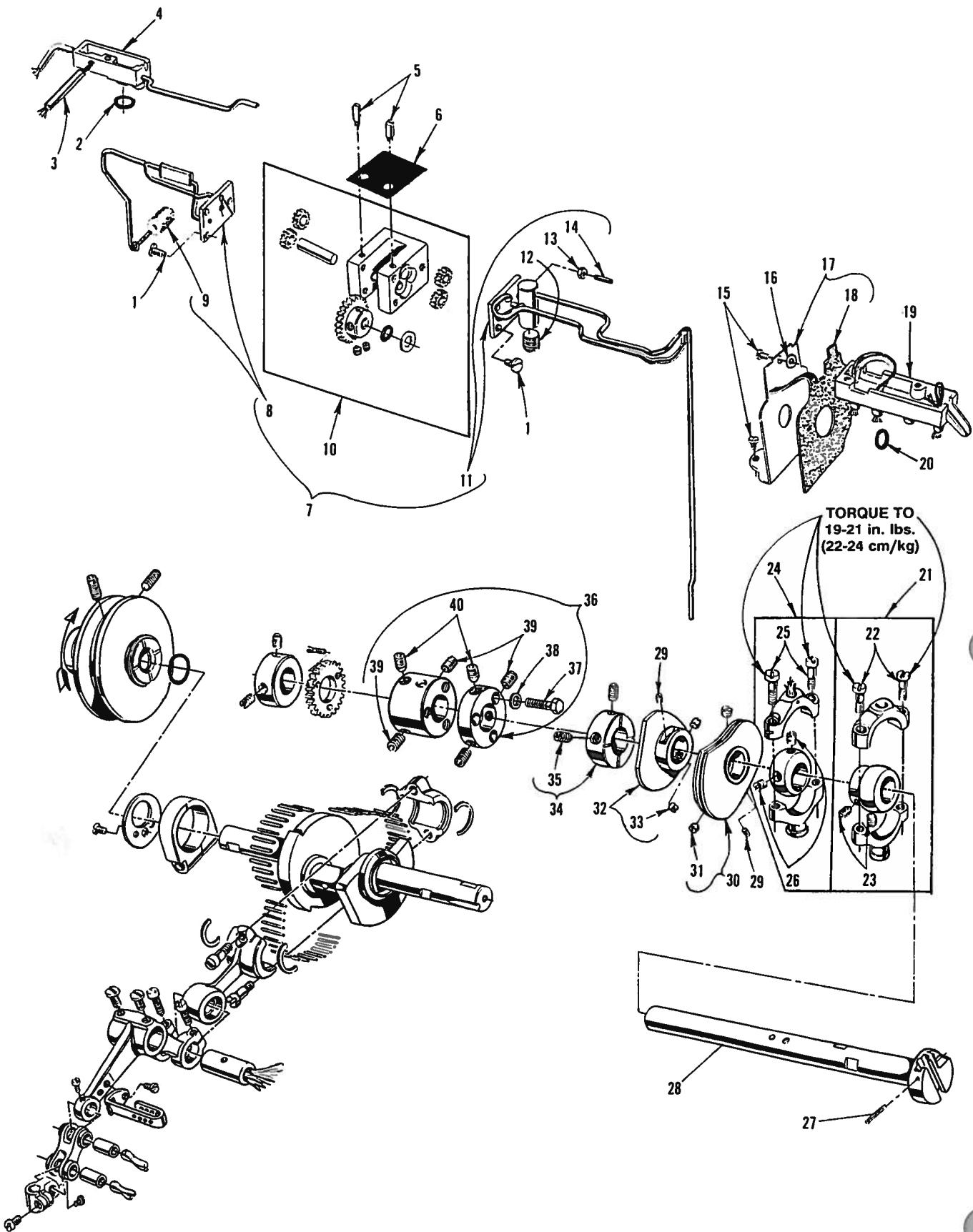
**MAIN SHAFT PARTS & MISCELLANEOUS OILING**
